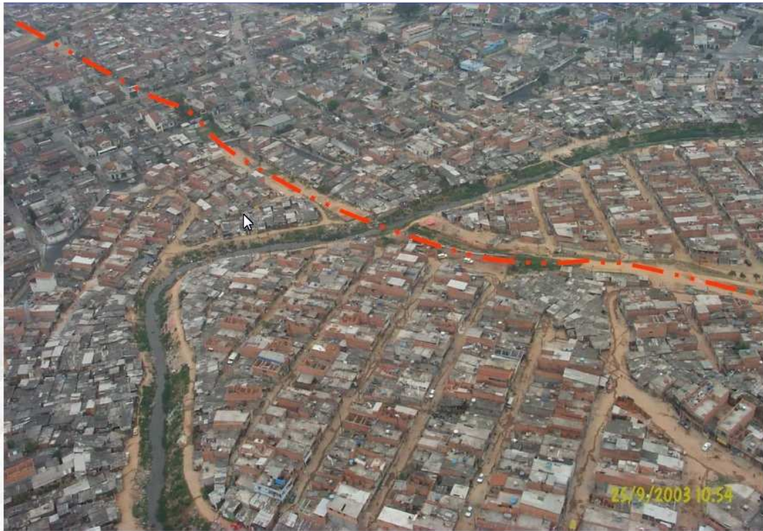
Figure 3.6 - Encroachment around the pipeline right-of-way. Reproduced from Petrobras/TRANSPETRO (Rennó retrieved April 2010)
