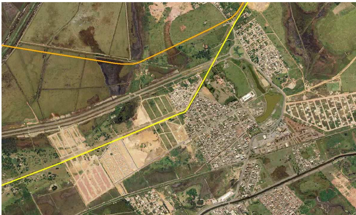
Figure 3.10 – City of Macaé, aerial photo taken in 2007 (scale 1:10,000). The yellow line is the pipeline right-of-way. The orange line is a proposed path to avoid the new urban development. Source: PETROBRAS/ENGENHARIA/IETEG/ETEG/EAMB - Engenharia de Avaliação Ambiental.
