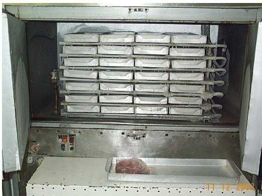
Figure 19 - Freezing in plate cabinets at -25 to -40°C.
